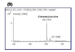
**Figure 1.** AccuTOF-DART<sup>TM</sup> Spectra of an Illicit Cocaine Sample Showing the Presence of: (A) Cocaine, Anhydroecgonine Methyl Ester (AEME), and Dimethylphthalate; and (B) Cinnamoylcocaines.
