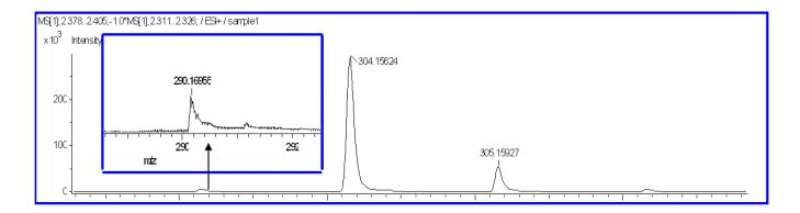
**Figure 2.** AccuTOF-Dart<sup>TM</sup> Spectra of an Illicit Cocaine Sample Showing the Presence of Possible Norcocaine and Benzoylecgonine (both at m/z = 290.17; see Expansion Window).
