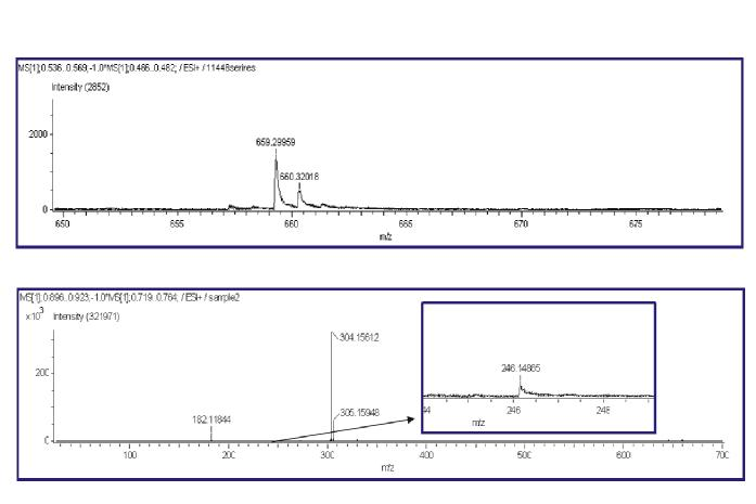
**Figure 3.** AccuTOF-DART<sup>TM</sup> Spectra of an Illicit Cocaine Sample Showing the Presence of: (A) Truxillines; and (B) Tropacocaine (in Expansion Window).
