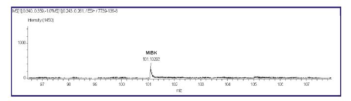
**Figure 4.** AccuTOF-DART<sup>TM</sup> Spectra of an Illicit Cocaine Sample Showing the Presence of: (A) Methyl Ethyl Ketone (MEK); and (B) Methyl Isobutyl Ketone (MIBK).
