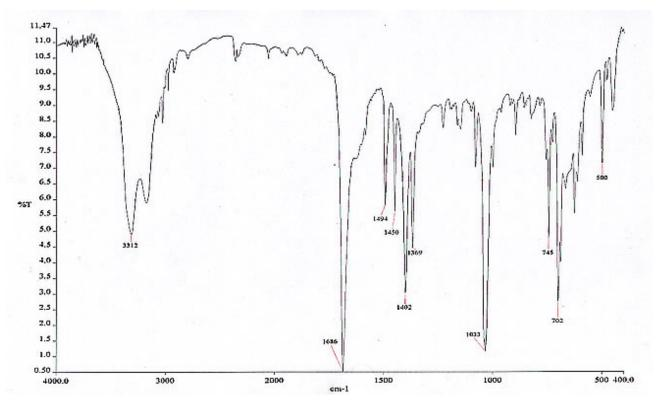
Figure 3 – Infrared Spectrum of Neat Modafinil
