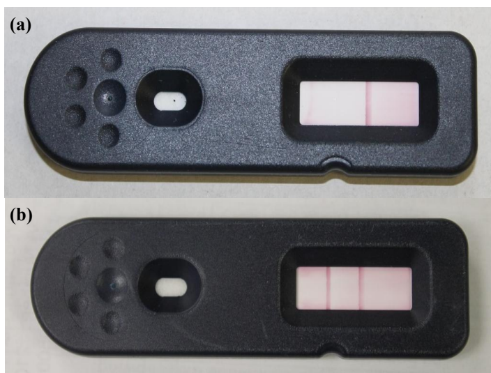
Figure 2 - Cozart ® cocaine solids test: (a) Positive test for cocaine, (b) Negative test for cocaine.
